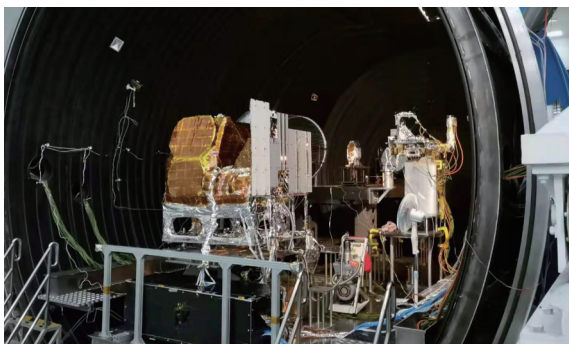
图9 热红外相机真空成像测试照片 Fig. 9 Vacuum imaging test picture of the thermal infrared camera
