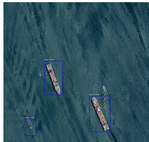
(c) 谷歌卫星影像的检测结果 (c) Test result from Google satellite imagery
