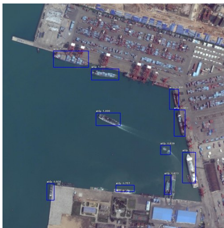
(c) 谷歌卫星影像的检测结果 (c) Test result from Google satellite imagery
