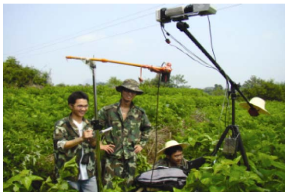
Fig. 8 Photograph of the FISS being used in the field
